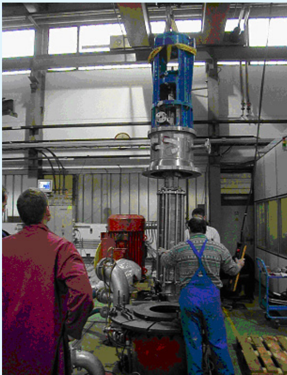
Installation of the centrifugal pump for a test run at the test-bench
